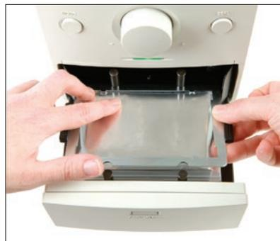
3. Place seal frame on sealing film.
