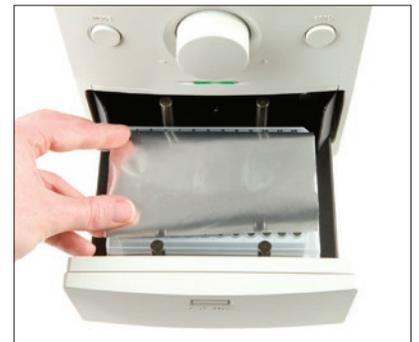
2. Place sealing film on plate.
